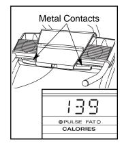
hands. When your pulse is detected, the Pulse indicator will light and then your heart rate will be shown in the main display. For the most accurate heart rate reading, continue to hold the contacts for about 15 seconds.
